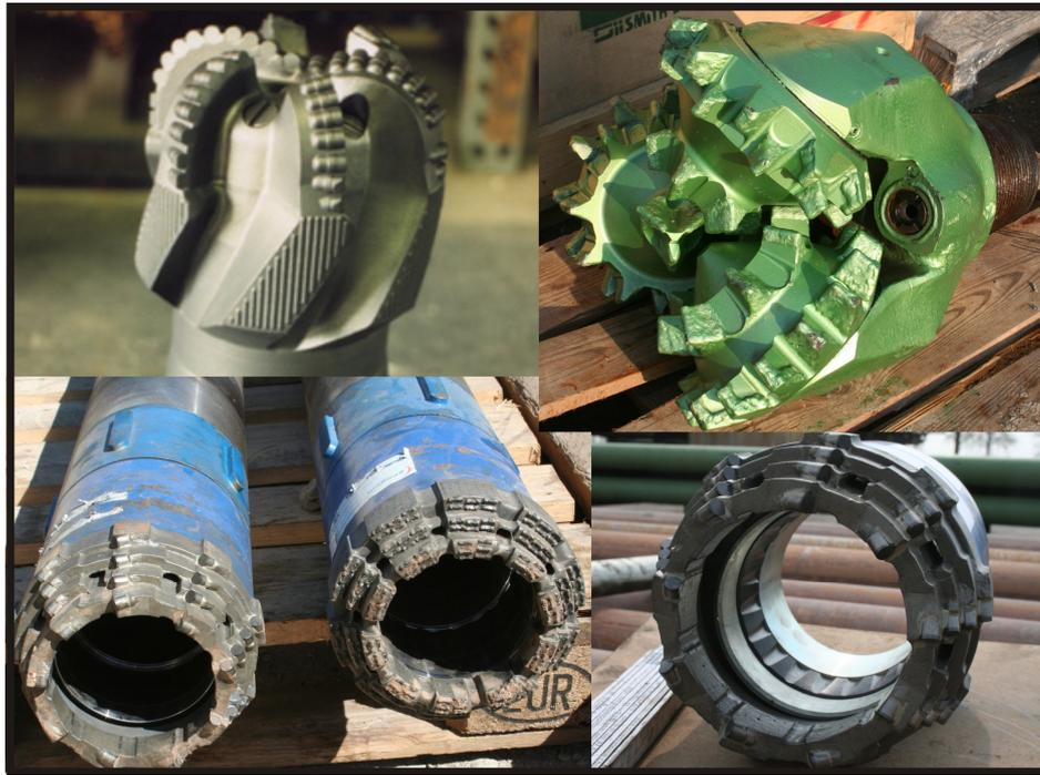
Figure 20: Drill bits (PDC bit, roller bit, and different core bit units (Photos by B. Norden)
