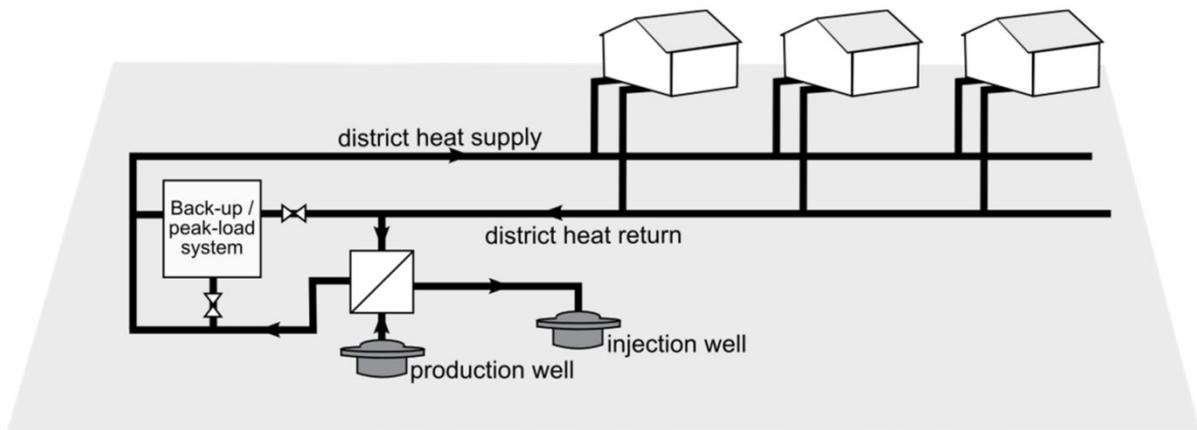
Figure 4: Scheme of a well doublet with back-up/peak-load system feeding a district heating grid
