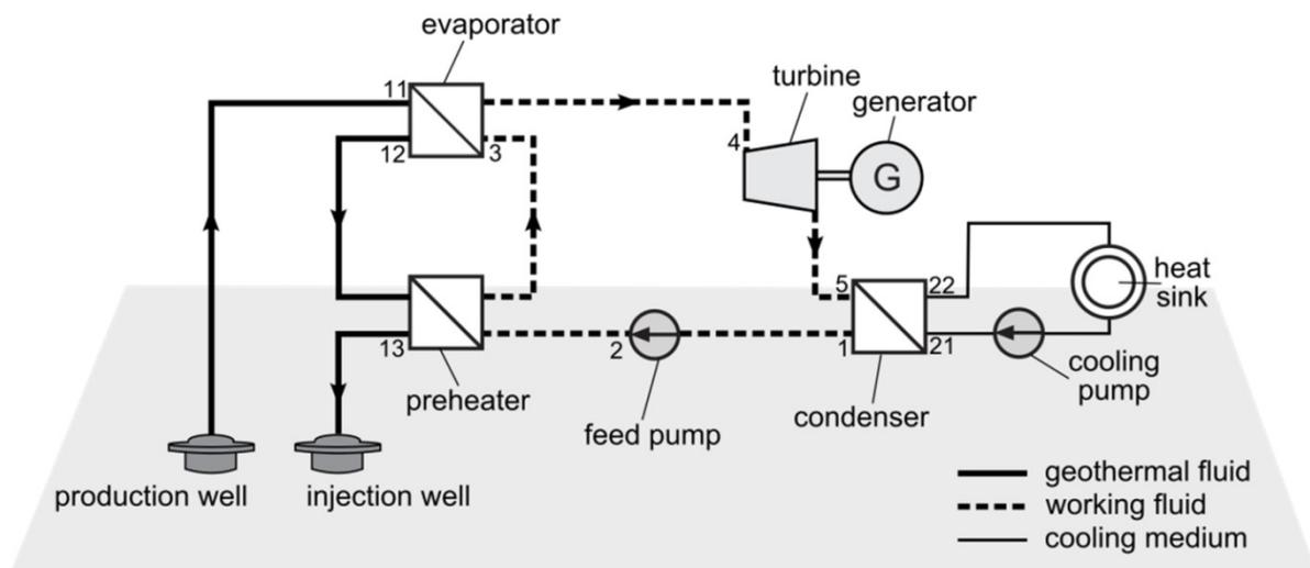
**Figure 8: Schematic set-up of Rankine cycle using geothermal heat as heat source**
