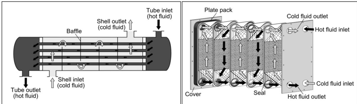
**Figure 17: Illustration of a shell-and-tube heat exchanger (left) and a plate heat exchanger (right)**
