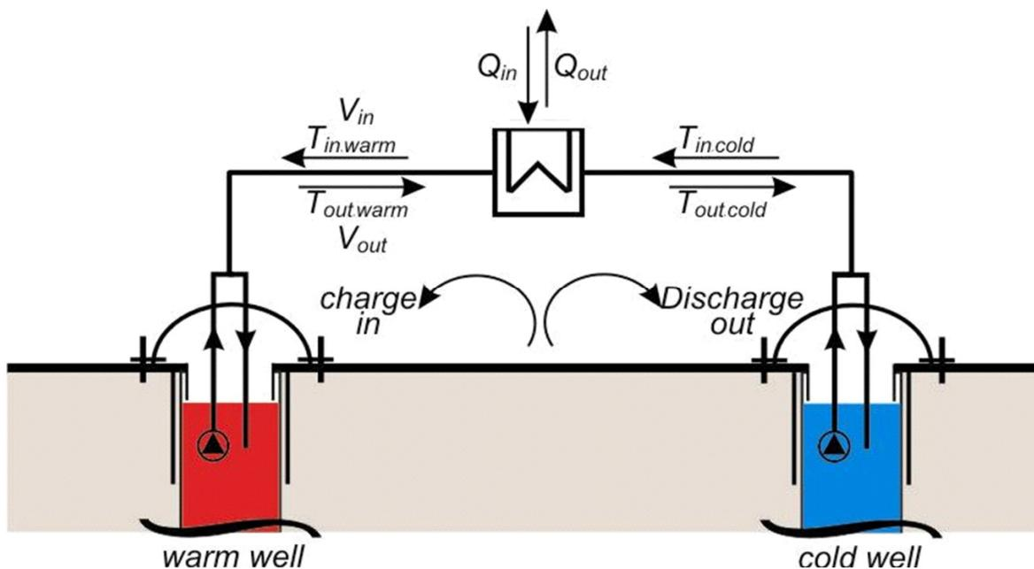
Figure 3: Scheme of an ATES doublet and notation
