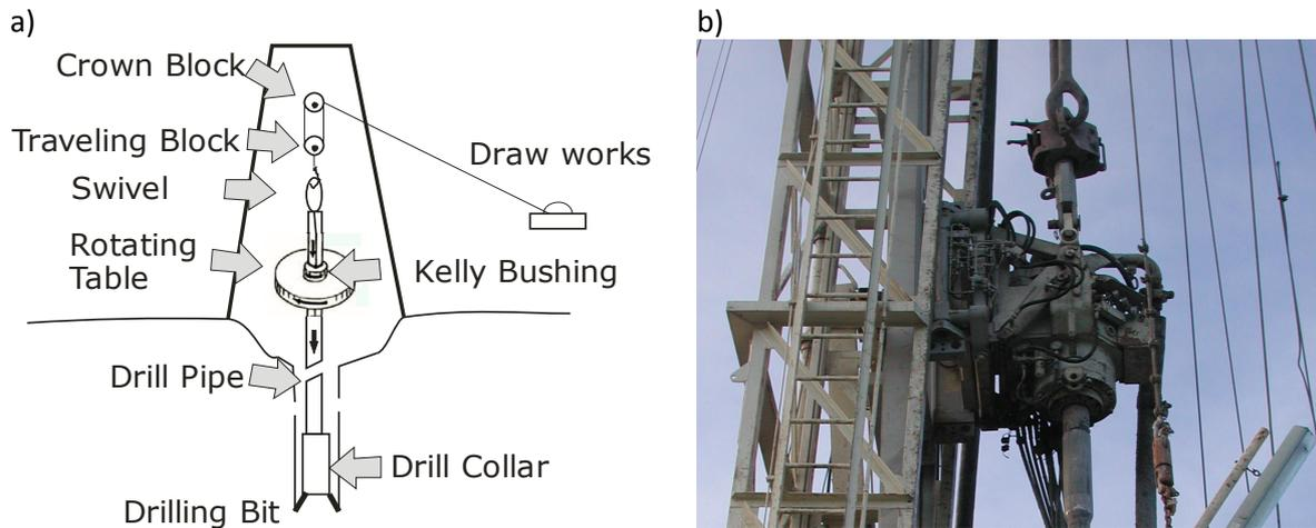
Figure 18: Rotary drilling. a) Rotary Table , b) Top Drive (Photo by B. Norden).
