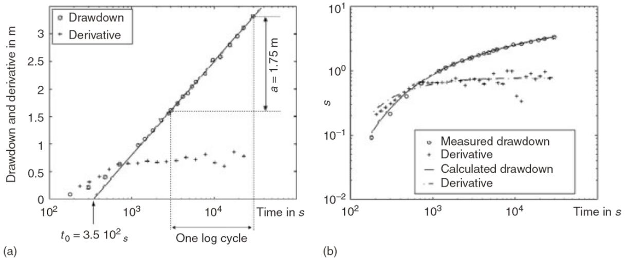
**Figure 23: Interpretation of a well-test data set with the Theis method. (a) semilog plot of drawdown and derivative; (b) superposition of the data with the model after automatic fitting (Renard, 2005)**
