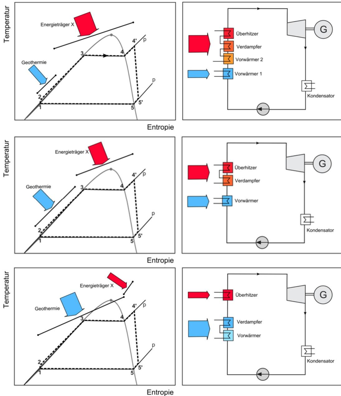
Figure 13: Temperature-Entropy Diagrams of a potential hybrid power plant. The relative input of geothermal energy increases from the concept at the top to the concept at the bottom.
