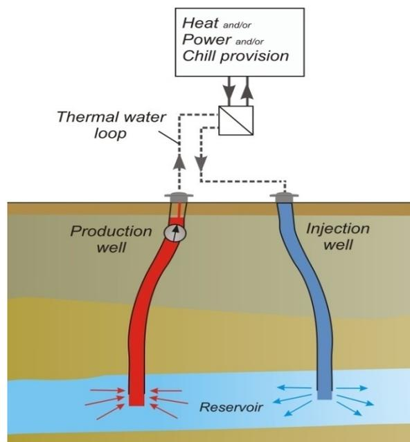
Figure 2: Principle for using a geothermal reservoir as heat source showing a well doublet, the geothermal fluid loop and a heat exchanger on the surface
