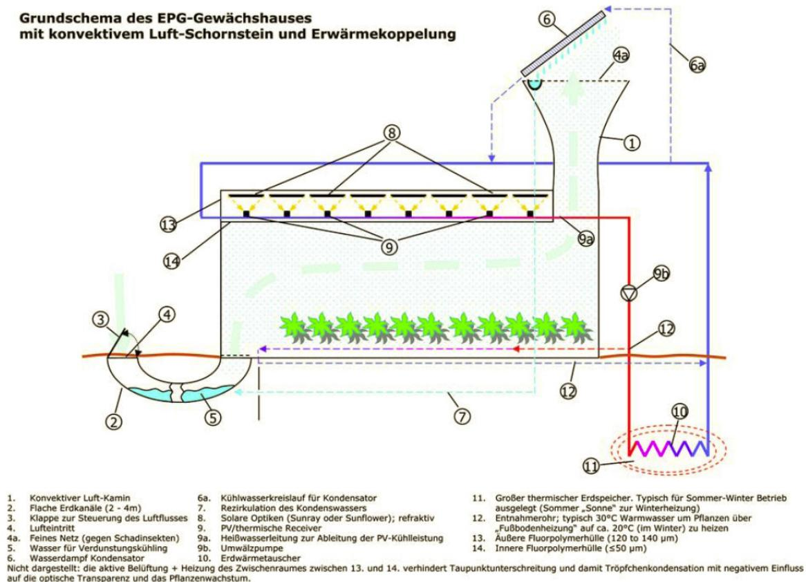
Figure 36: Sketch of a greenhouse using solar heat and underground thermal storage (Kleinwächter et al., 2006)
