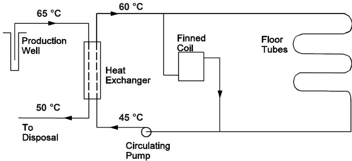
Figure 35: Example of a greenhouse heating system (modified from Rafferty, 1998)
