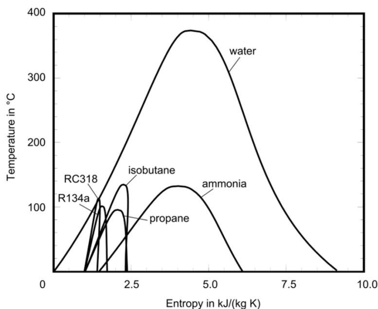
Figure 9: Temperature-entropy diagram showing the saturation vapour curves of different working fluids
