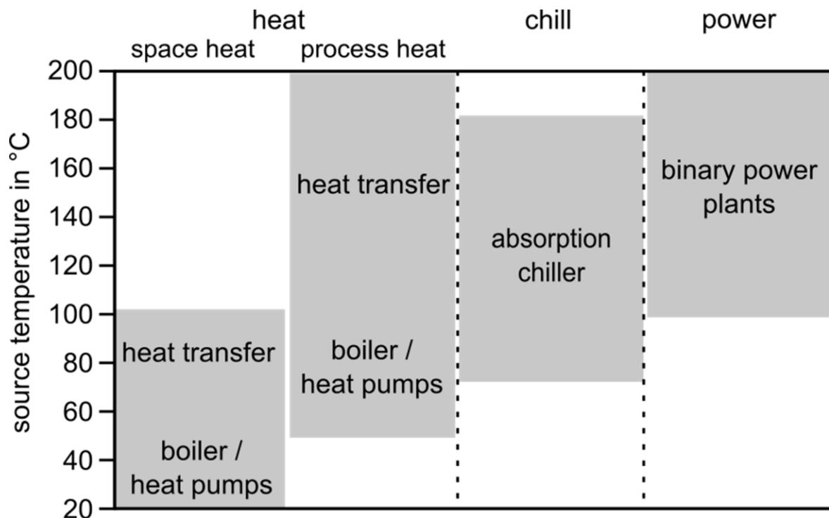
Figure 1: Energy supply options with different plant technologies from heat sources with temperatures between 20 and 200 °C derived from Lindal (1973)
