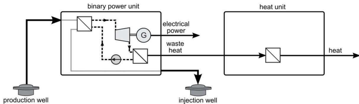
Figure 11: Schematic set-up of a plant with conventional cogeneration of power and heat
