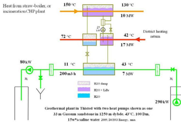
Figure 31: Geothermal plant in Thisted (Mahler & Magtengaard, 2010)
