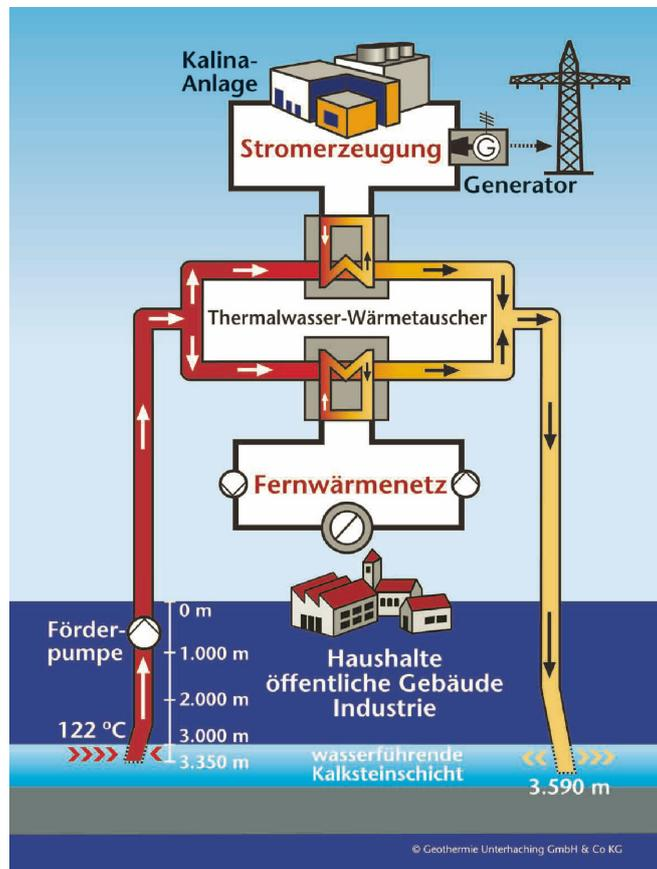
Figure 34: Scheme of the Unterhaching geothermal plant
