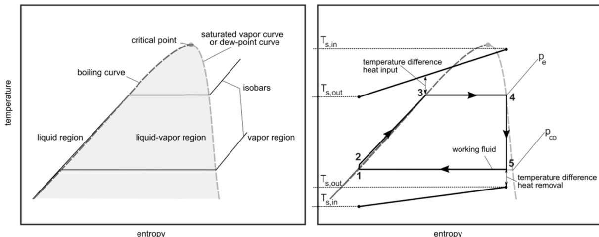
Figure 7: Temperature-entropy-diagram (T-s diagram) of an example working fluid showing general notations (left) and a corresponding Rankine cycle with saturated vapor (right)
