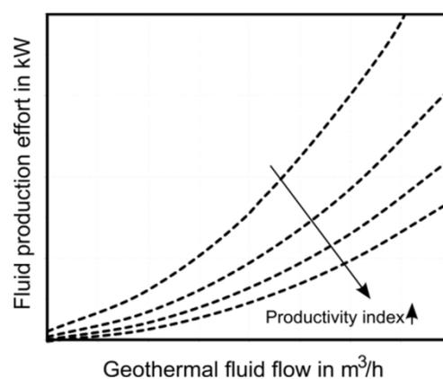
**Figure 16: Qualitative development of fluid production effort as a function of geothermal fluid flow for different reservoir productivities**
