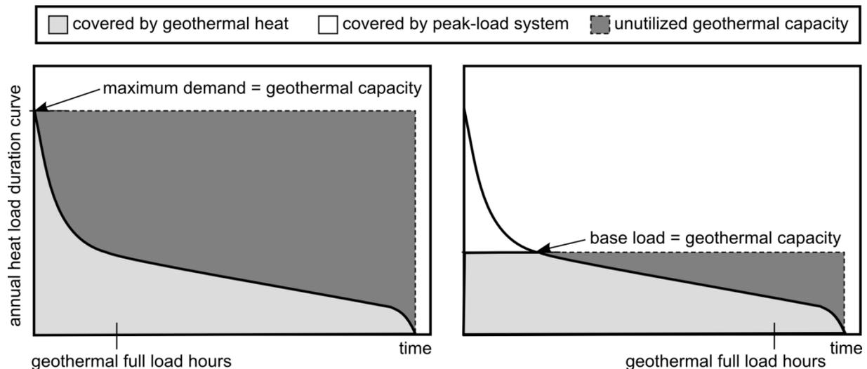
Figure 5: Annual heat load duration curves and corresponding geothermal plant design
