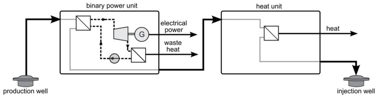
**Figure 12: Schematic set-up of a geothermal plant with power and heat supply in serial connection**
