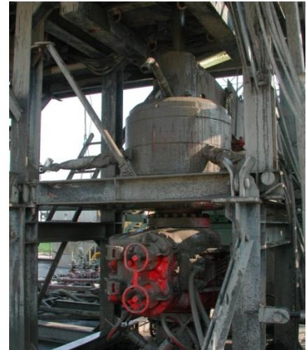
Figure 19: Blowout preventer unit of a drill rig in Ketzin (Photo by B. Norden)
