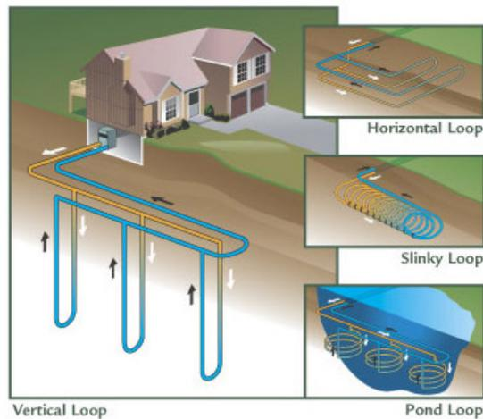
Figure 29: Geothermal heat pump installation systems (Reference: [www.architecture2030.org](http://www.architecture2030.org), 19-05-2010)
