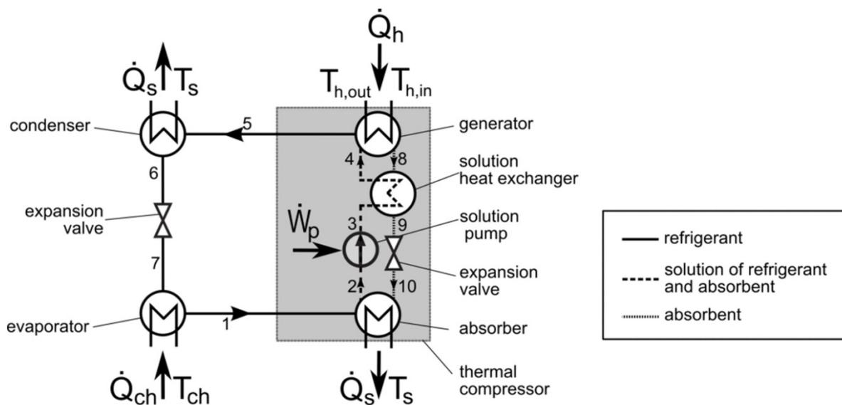
Figure 6: Principle of an absorption refrigeration cycle
