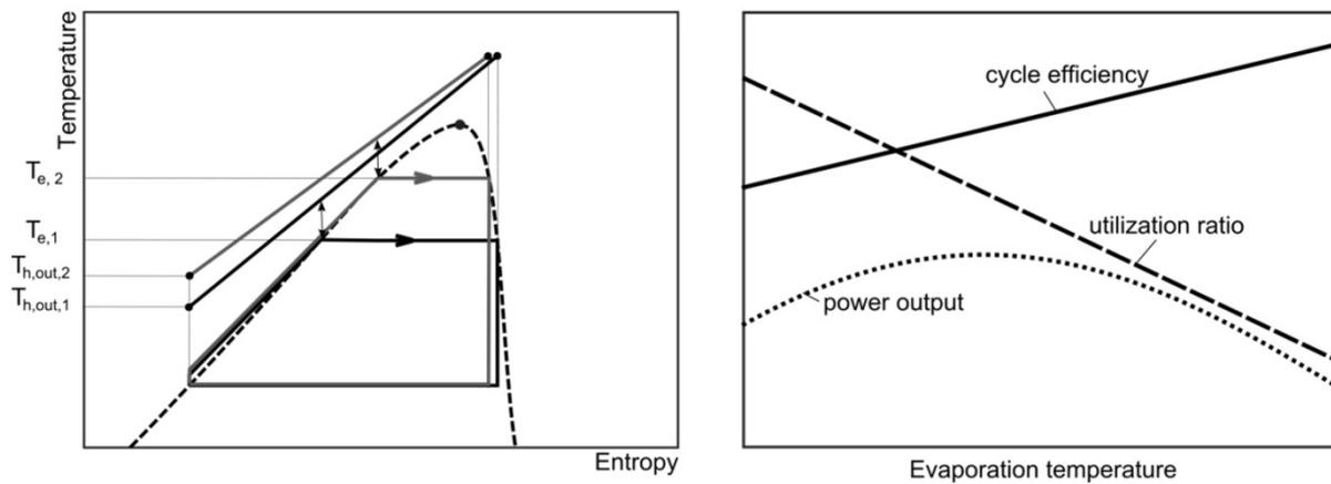
**Figure 10:** T-s diagram showing the correlation of evaporation temperature and geothermal outlet temperature (left) and development of power output as a function of the evaporation temperature (right)
