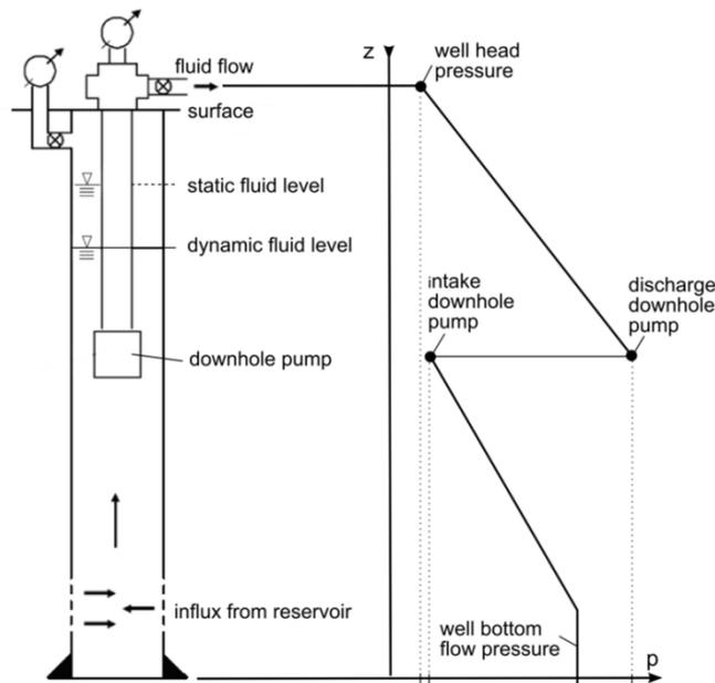
**Figure 15: Scheme of a production well showing downhole pump, static fluid level and dynamic fluid level (left) and the pressure curve during fluid production (right)**
