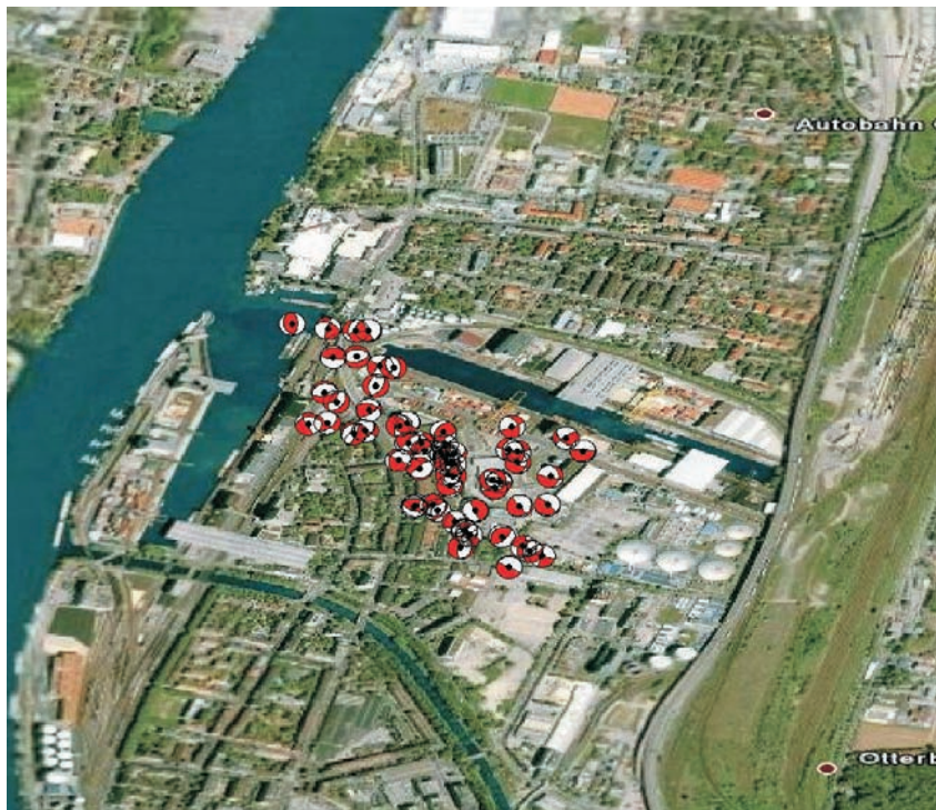
Figure 1. Air photo showing location of induced earthquake beneath the Basel HDR site.
