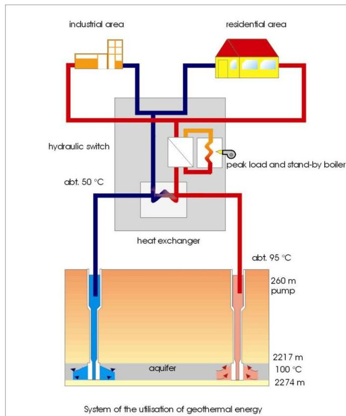
FIGURE 2.3: A scheme of the Neustadt-Glewe geothermal space-heating plant, Germany (Menzel et al., 2000)
