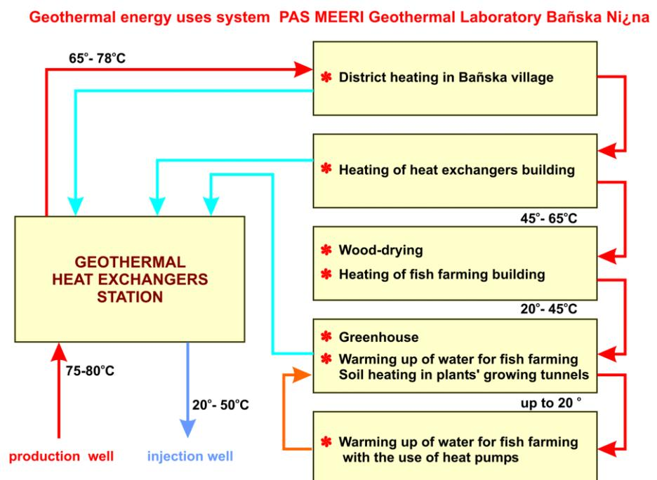
FIGURE 4.14: Sketch of cascaded uses system, PAS MEERI Geothermal Laboratory
