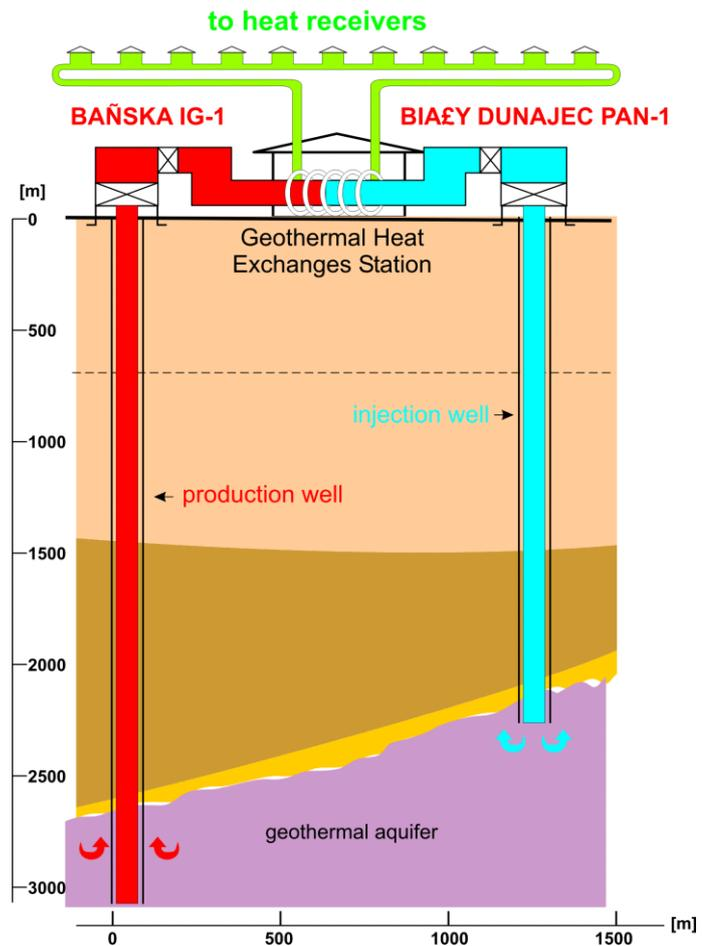
FIGURE 4.7: Sketch of the geothermal doublet working from 1992-2001, PAS MEERI Geothermal Laboratory
