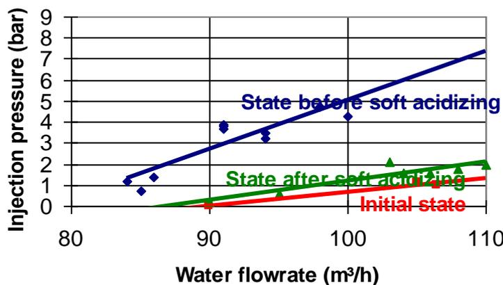
FIGURE 2.4: The Neustadt-Glewe geothermal space-heating plant, Germany – soft acidizing results shown by significant lowering of the injection pressure (Menzel et al., 2000)
