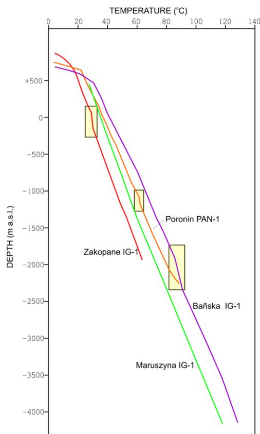
FIGURE 4.4: Temperature logs from some wells drilled within the Podhale region. Marked is a blanket effect in caprock of main geothermal aquifer (Kepinska, 2000)
