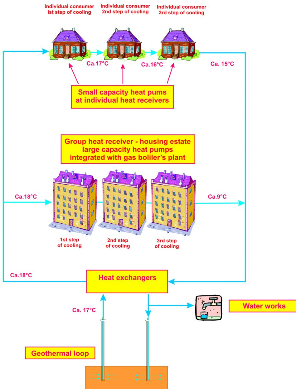
FIGURE 3.7: A sketch of a geothermal plant in Slomniki
