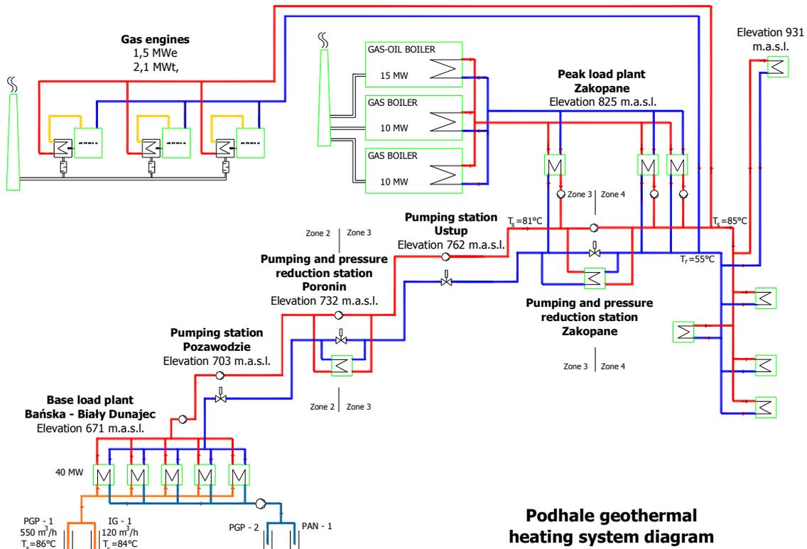
FIGURE 4.8: Technical diagram of the geothermal heating system under construction in the Podhale region (Dlugosz, 2003)
