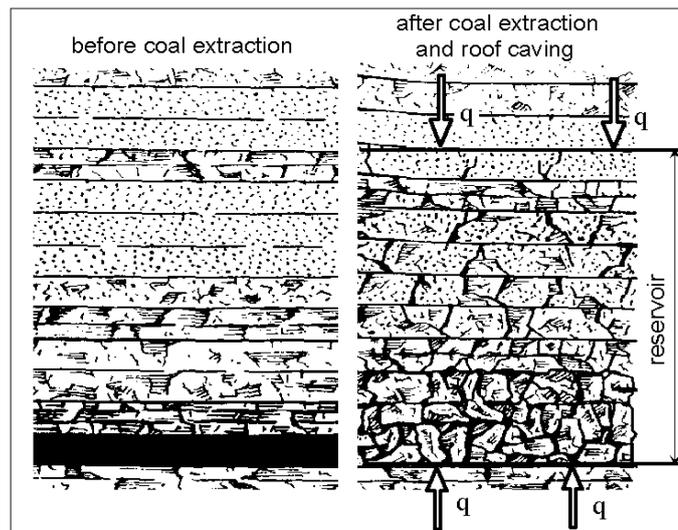
FIGURE 2.6: Sketch of water reservoir in the mine workings after extraction of coal seam (black layer) and caving in of the roof; arrows  $q$  mark heat inflow (Malolepszy, 2003)
