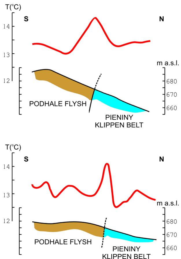
FIGURE 4.5: Surface thermal anomalies above the tectonic contact zone between the Podhale geothermal system and the Pieniny Klippen (according to Pomianowski, 1988)
