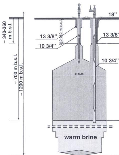
FIGURE 2.10: A sketch of a chamber formed as a result of salt brine underground leaching method and used for underground storage (based on Bujakowski [ed.] et al., 2003)
