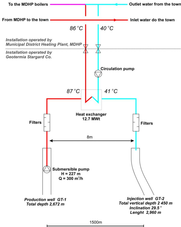
FIGURE 3.8: Stargard Szczecinski - a sketch diagram of a geothermal plant (Kozłowski and Malenta, 2002)
