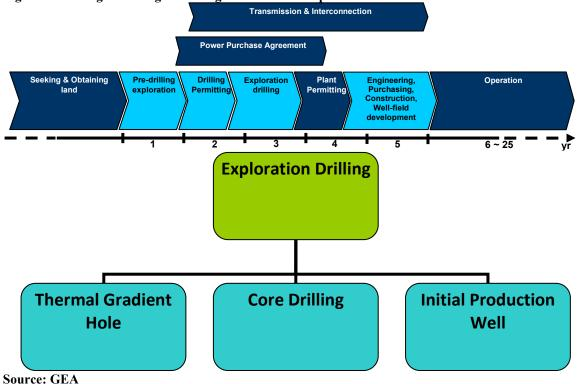
Figure 3: Drilling technologies in the geothermal development timeframe
