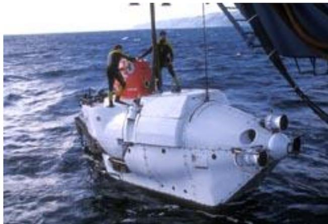
Figure 33) Launching of the submersible Alvin [80].
