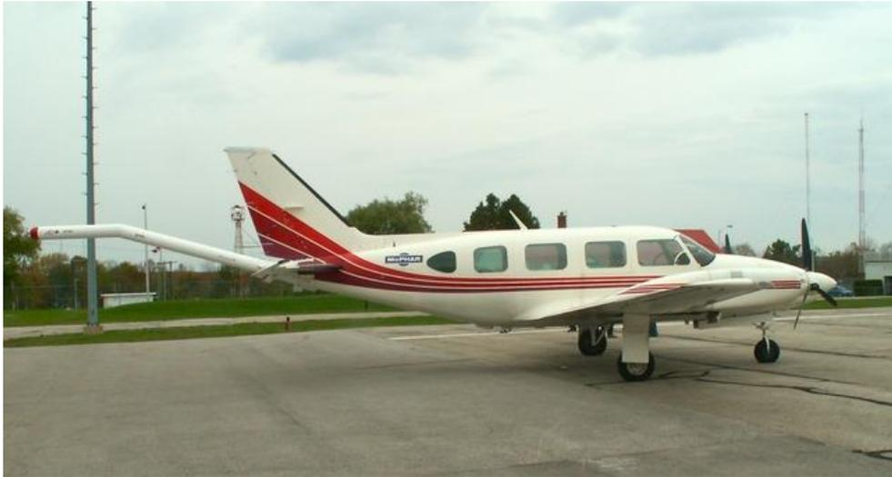
**Figure 38) A total field magnetometer installed onto the back of an aircraft [89].**
