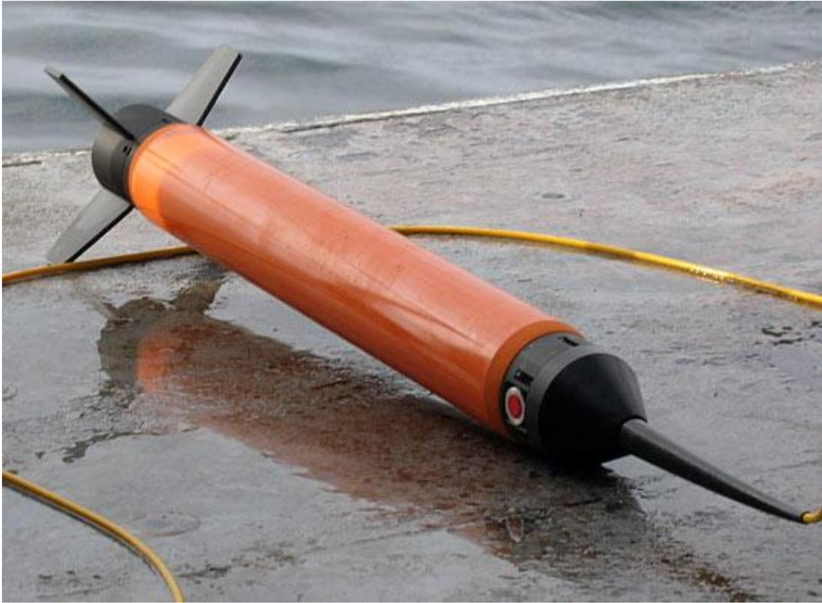
Figure 39) Marine magnetometer; this instrument is about 2 meters in length and is towed by a cable. While in tow the instrument transmits magnetic measurements to a computer onboard the ship [91].
