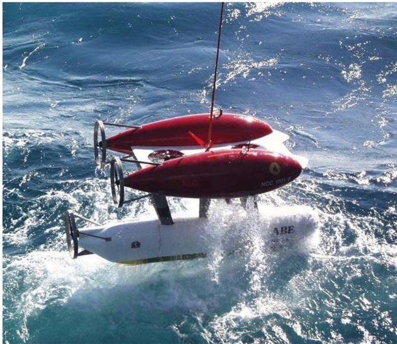
**Figure 35) An AUV being deployed for hydrothermal vent exploration [81].**
