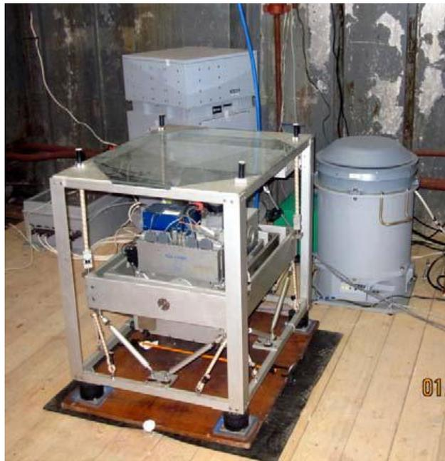
Figure 41) Marine gravity meter [92]
