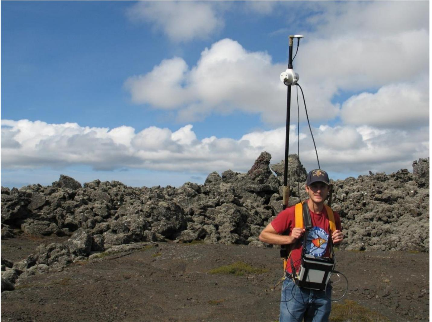
Figure 37) Equipment used for a ground magnetic survey. The magnetometer is on a pole roughly 2.5 meters above the ground. A GPS is at the very top of the pole. The computer is strapped around the stomach.
