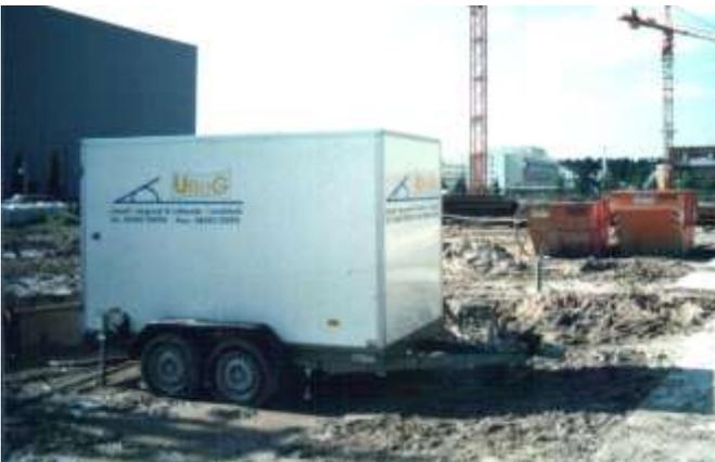
Figure 2: The first UBeG TRT-rig: left for the first TRT done in Germany in 1999 (Sanner et al. 1999), right with a generator at a site without electricity)
