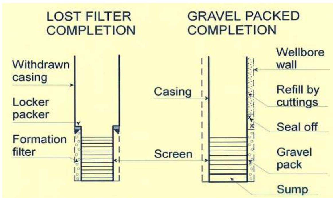
Fig. 4. The two main types of screened wells and their principal design and components
