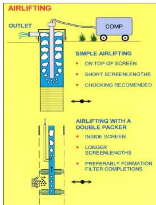
**Easy and practical to arrange if the well has been drilled with air**
