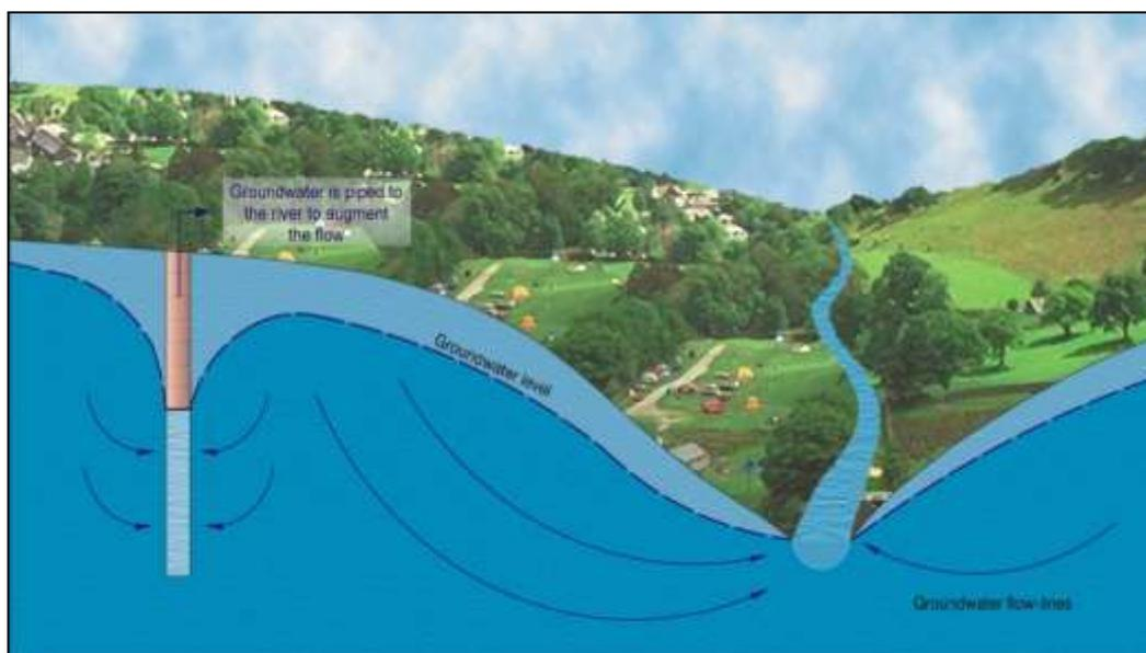
Figure 3. The flow of groundwater in an unconfined aquifer, in this case partly to a river and partly to a water well.
