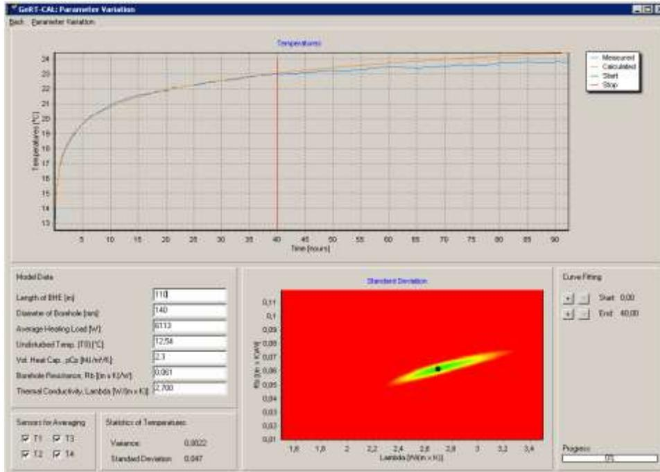
Figure 11: Parameter variation for TRT data (search for the “best fit”), with a linear area of good fit (green area)
