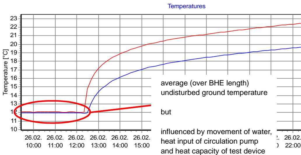
Figure 12: Measurement of undisturbed ground temperature by water circulation without heating
