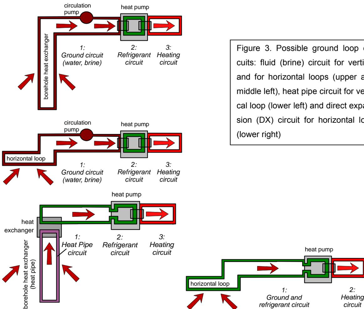
Figure 3. Possible ground loop circuits: fluid (brine) circuit for vertical and for horizontal loops (upper and middle left), heat pipe circuit for vertical loop (lower left) and direct expansion (DX) circuit for horizontal loop (lower right)
