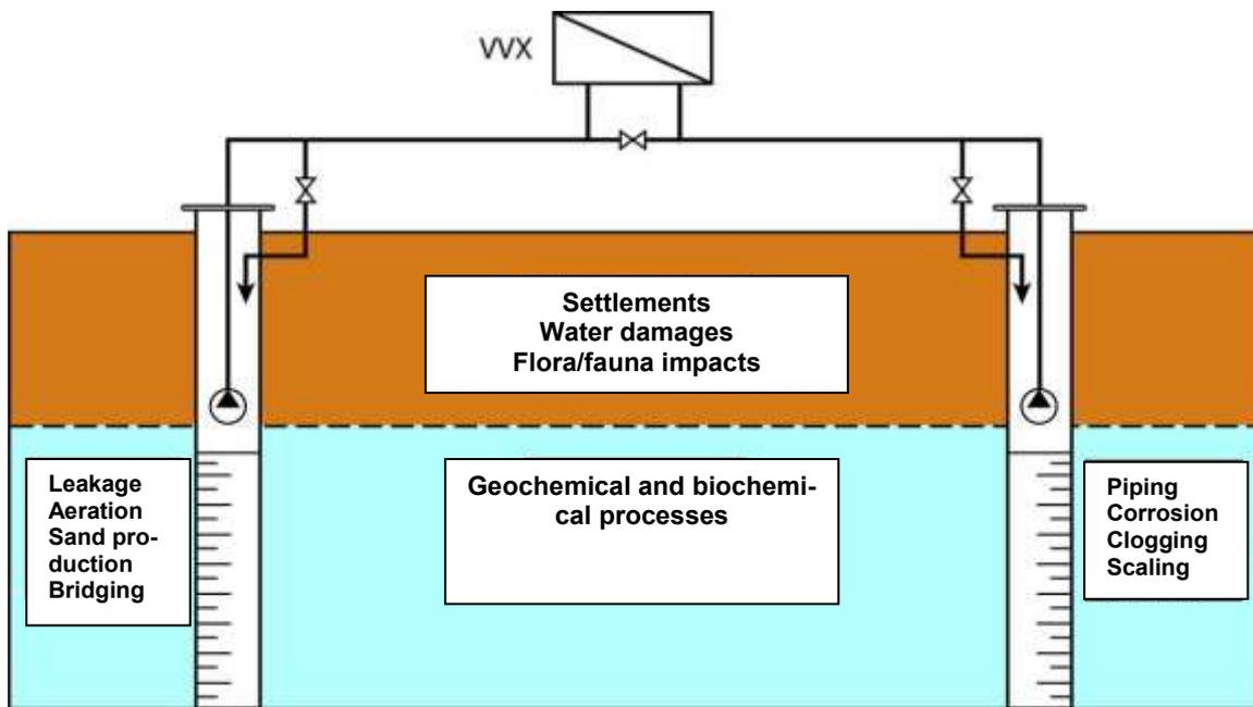
Fig. 1. Potential technical and environmental problems related to open loop systems
