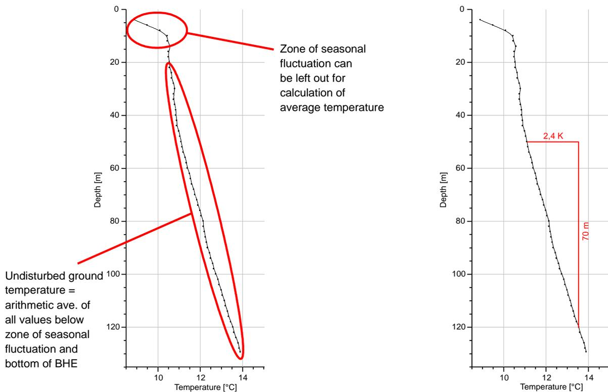
Figure 14: Temperature log and evaluation of average undisturbed ground temperature (left) and geothermal gradient (right, see text)
