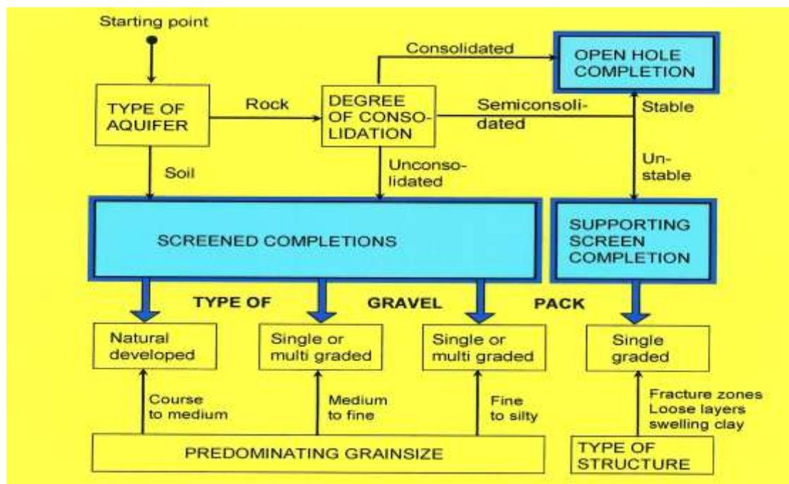
Fig. 11 Flow chart for selection of well type based on geological conditions
