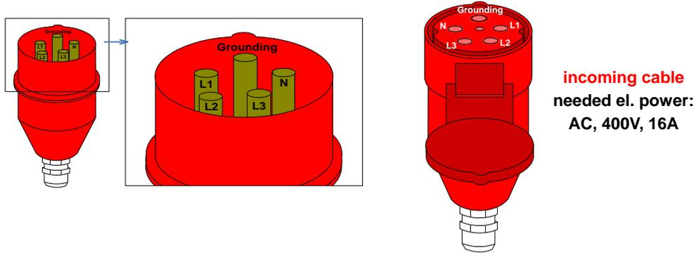
Figure 7: Before connecting the TRT to the power supply, check the phases!
