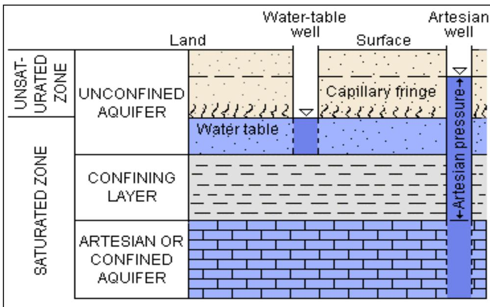
Figure 2. The types of aquifers unconfined with a free groundwater table and confined with a static head (artesian pressure).
