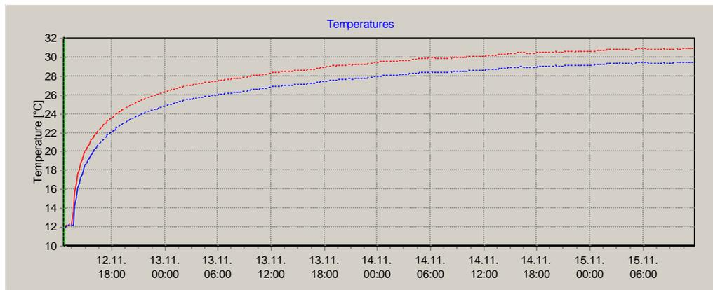
Figure 1: Principle of a TRT and temperature curve of inlet-outlet (good example)
