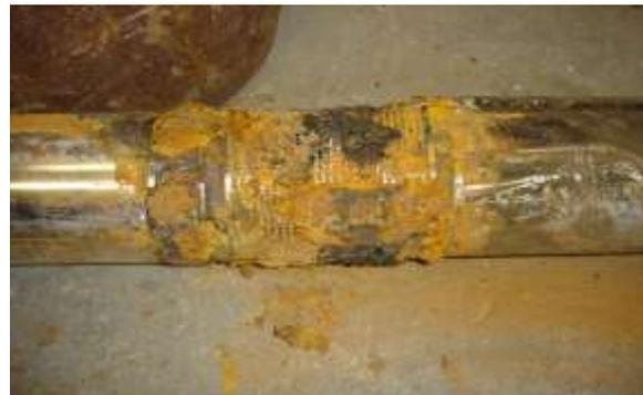
**Clogging is defined as an “increased resistance for the water to enter the well”, and it will result in:**
