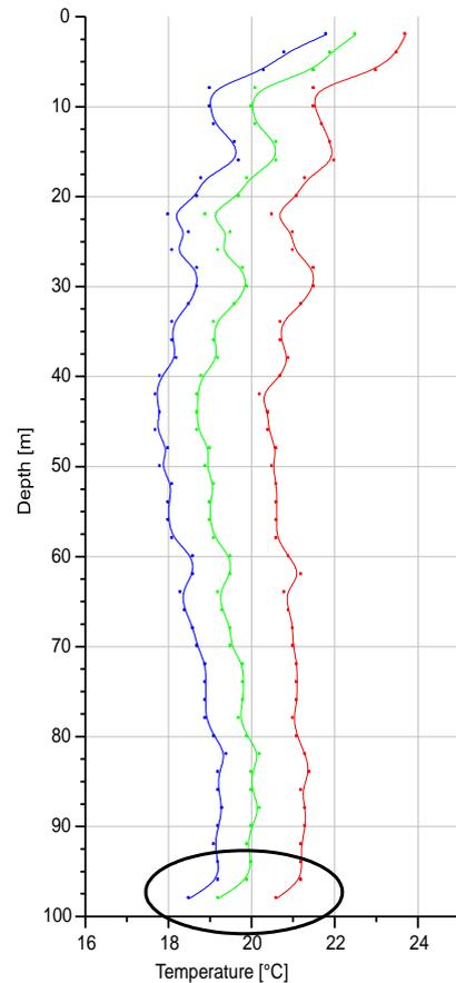
Figure 15: Features as elucidated by temperature log before and after TRT: Influence of groundwater-flow (top left), poor or non-existent grouting (top right), presence of a low-conductivity layer (bottom left), prove of final depth (bottom right)
