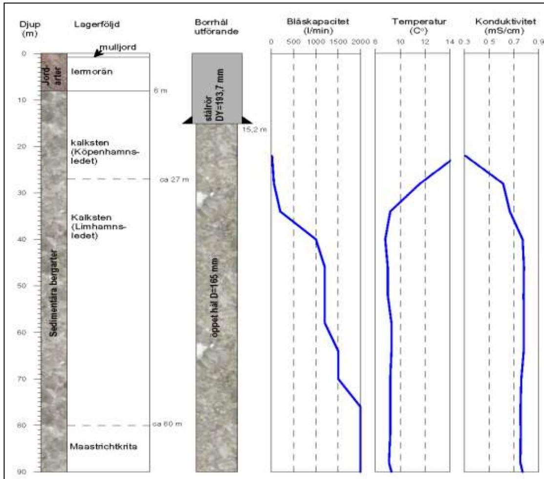
Fig 5. Results from a test drilling for an ATEs plant in limestone to IKEA Malmö, Sweden
