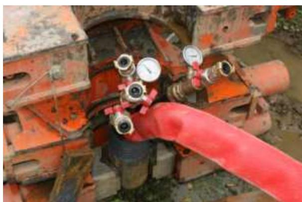
Figure 5. Cut the tubes to required length, fill them with water, apply a first pressure and seal them
