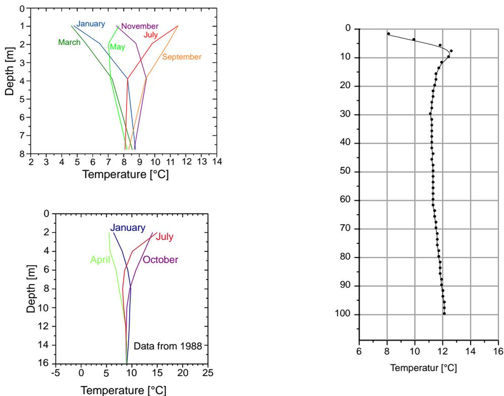
Figure 1. Constant temperature in the “Neutral Zone” at 10-20 m depth development, and temperature development down to 100 m depth (anticlockwise from top left):
