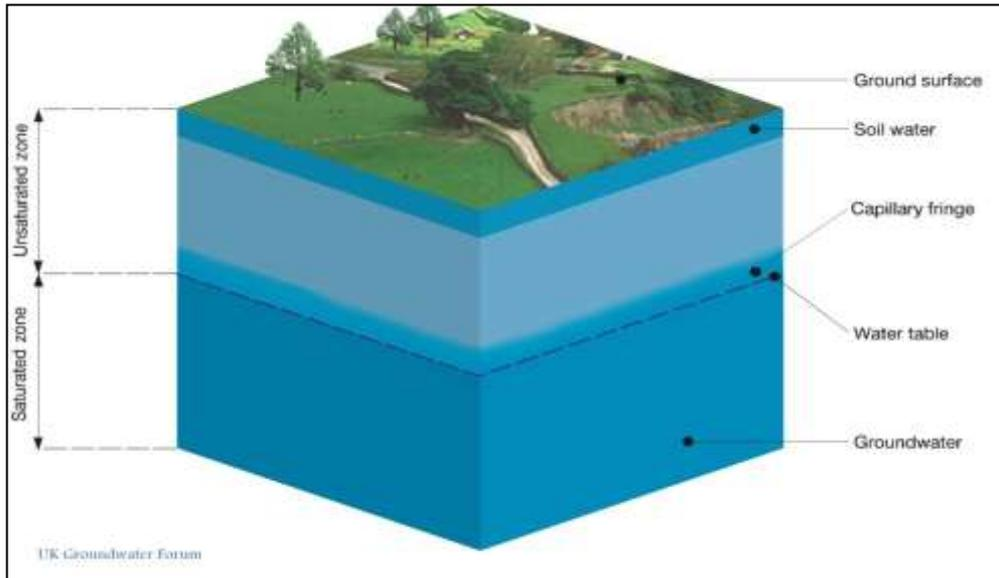
Figure 1. The saturated zone defines the groundwater table. An aquifer is in practice defined to be a limited geological formation from which ground water can be pumped by using water wells.
