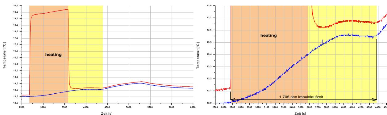
Figure 16: Principle of Thermo-Impulse method (recurrence of impulse)
