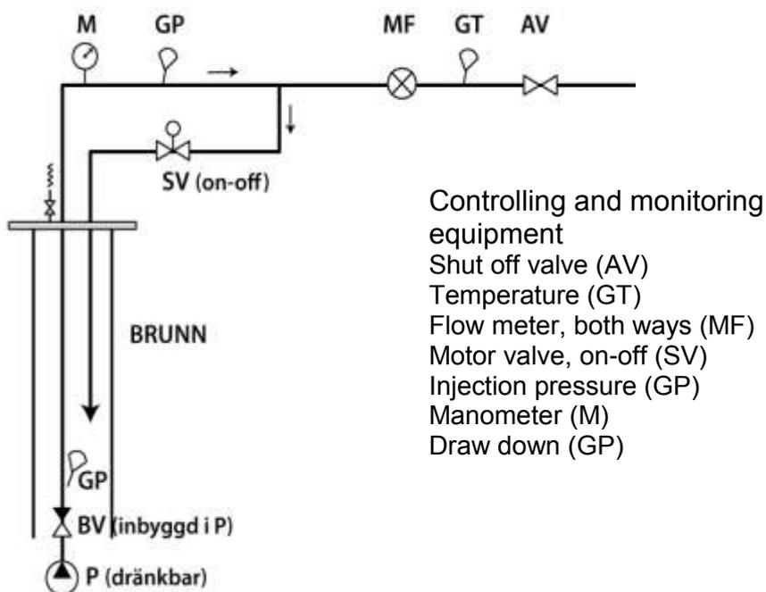
Fig. 2. Example of controlling and monitoring devices for wells used for both extraction and injection
