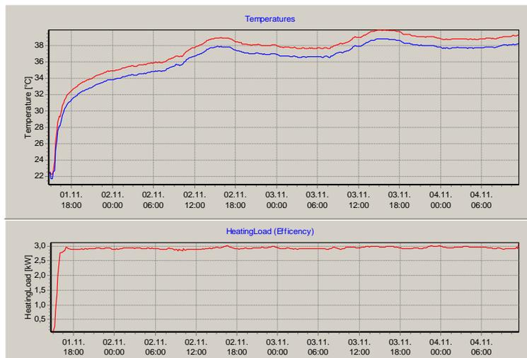
Figure 5: Result of inappropriate setup, with large temperature fluctuations at rather steady heat load
