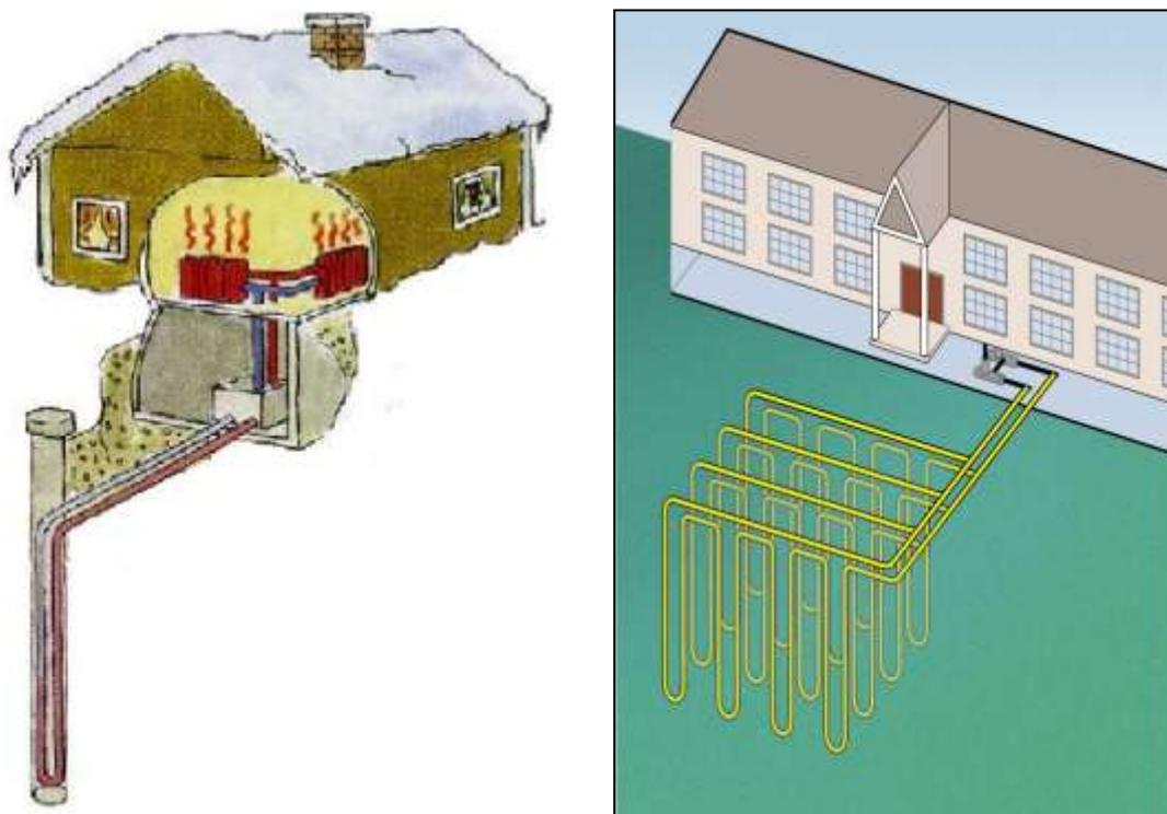
*Fig.2. Vertical closed loops applied for a single and a multifamily residential building*
