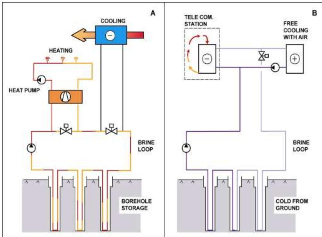
Fig.7. Principal system for combined heating and comfort cooling (A) and for process cooling (B)
