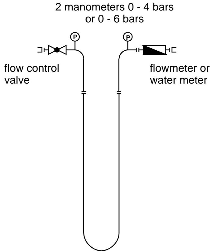
Figure 3. Flow test configuration (graph: Polydynamics Engineering Zurich)
