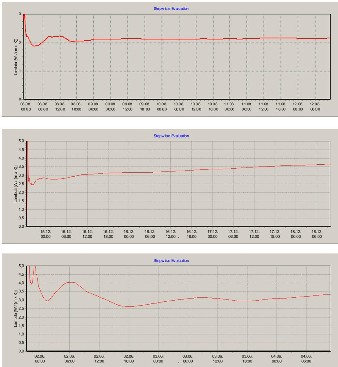
Figure 10: Examples of stepwise evaluation of TRT: Dominated by conductivity, good reliability (top), dominated by advection and not usable (middle), and high fluctuations and low reliability (bottom)
