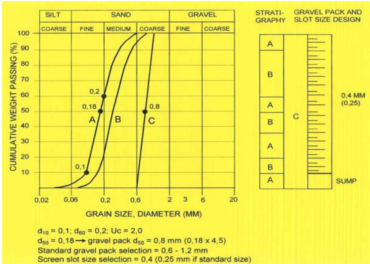
Fig.10. Example on how to select the gravel pack (C) and screen based on the grain size distribution of finest grained layer (A).
