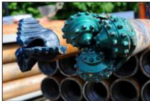
*Figure 4. Conventional rotary drilling and different bits used (a three cone roller bit and a drag bit).*
