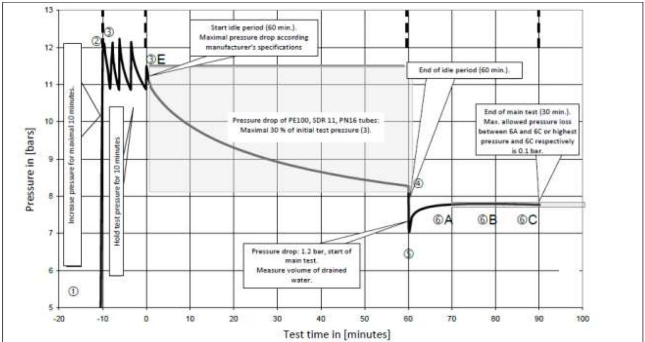
Figure 6. Graphical test procedure (graph from SIA 384/6 (SN 546 384/6)).
