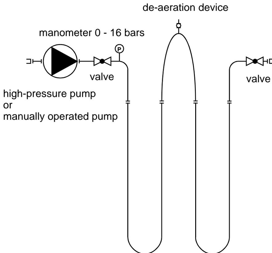
Figure 5. Leak tightness test configuration (graph: Polydynamics Engineering Zurich)
