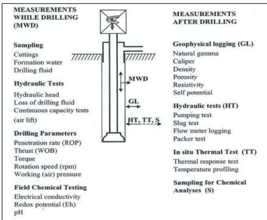
Fig 2. Potential parameters that can be achieved from a test drilling during and after drilling
