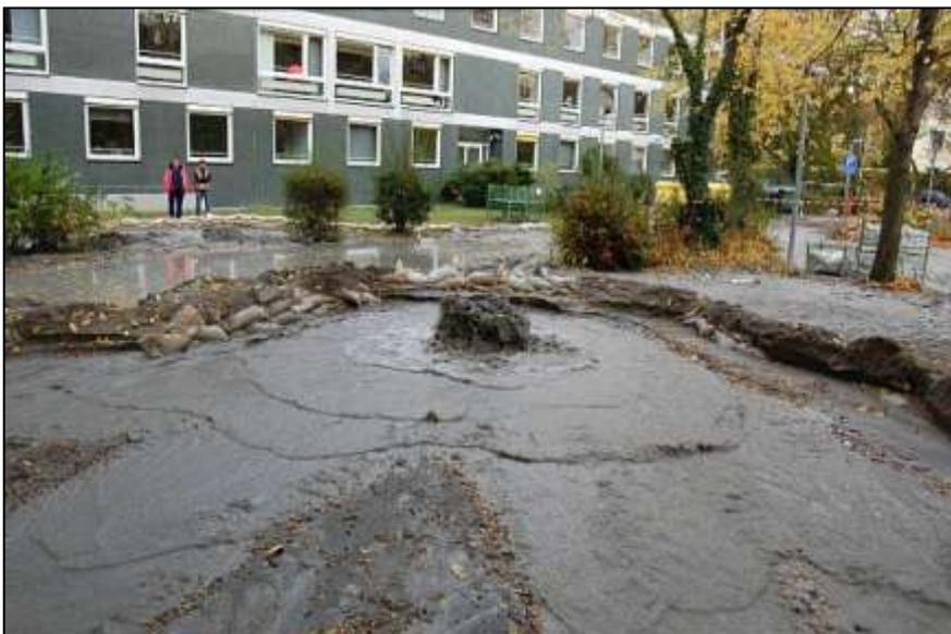
Figure 1. Example of artesian flow creating environmental problems
