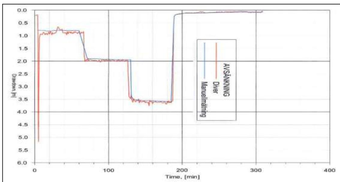
Fig.12. Example of step draw down test to determine the efficiency of a well.
