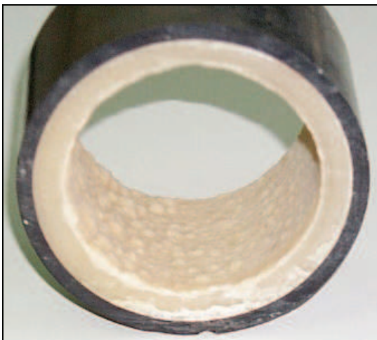
Figure 9.1. Pictures of scaled geothermal pipes. Left, \text{CaCO}_3 scales in a pipe carrying low-enthalpy geothermal water at Nigrita, Greece. Right, mixed silica and sulphide scales in the reinjection pipe of Milos geothermal plant.
