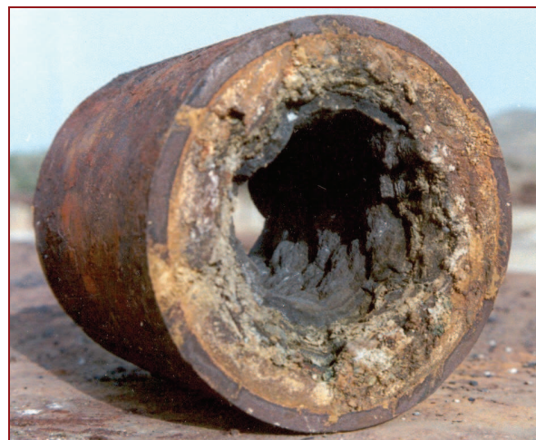
Figure 9.1. Pictures of scaled geothermal pipes. Left, \text{CaCO}_3 scales in a pipe carrying low-enthalpy geothermal water at Nigrita, Greece. Right, mixed silica and sulphide scales in the reinjection pipe of Milos geothermal plant.
