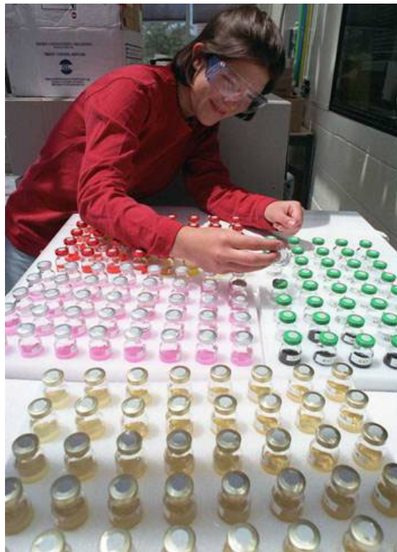
Figure 7. Examination of sample dilution vials of various cultures for MPN analyses.
