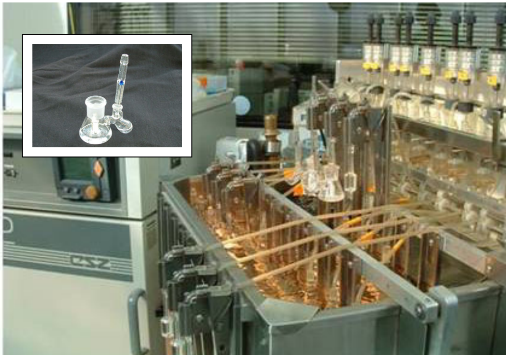
Figure 18. Gilson differential respirometer and close-up of 15 ml reaction flask.
