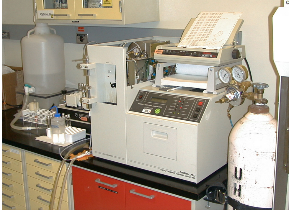
Figure 12. Total Organic Carbon Analyzer, OI Corporation (College Station, Texas).
