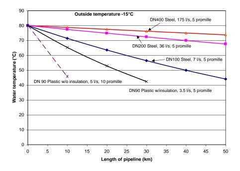
Figure 9 Examples of calculated temperature drop in pipelines. From top to bottom: Surface mounted steel pipeline, buried pre-insulated pipes and finally two examples of plastic (PP, PB) pipe with and without thermal insulation.
