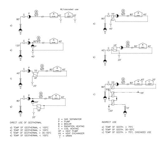
Figure 2 Examples of district heating network with geothermal water
