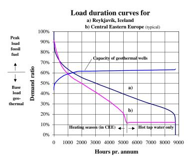
Figure 1 Typical load duration curves. Curve a) depicts a district heating system with a high load factor and b) system with a low load factor (no space heating during summer season.)
