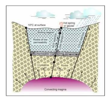
Fig 1: Schematic representation of high temperature hydrothermal reservoir
