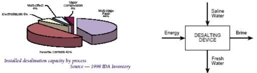
Fig 2: Installed desalination capacity (1998 left) and basic principle (right)
