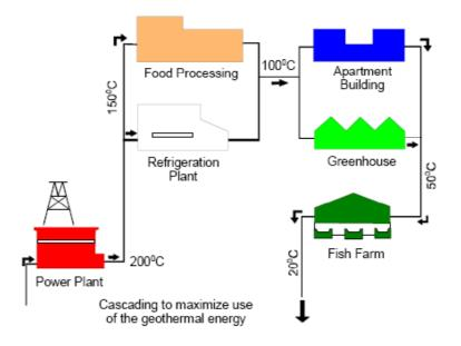
Figure 11. An example of geothermal cascading (combined heat and power).
