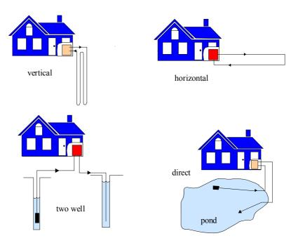
Figure 10. Typical closed and open loop geothermal heat pump installations.
