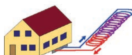
Compact ground heat exchangers (top: trench collector, bottom: slinky collector)
