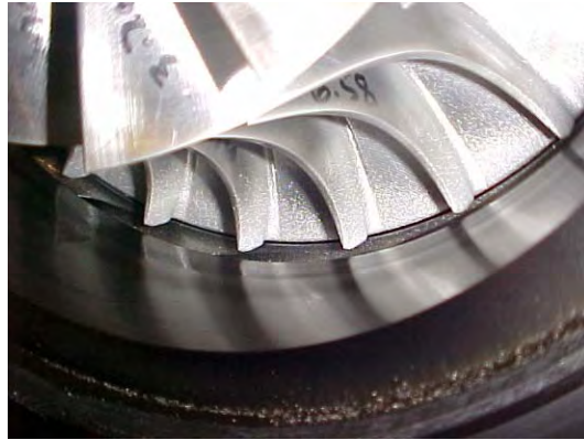
Figure 8. Turbine Impeller Erosion after qualification test in April
