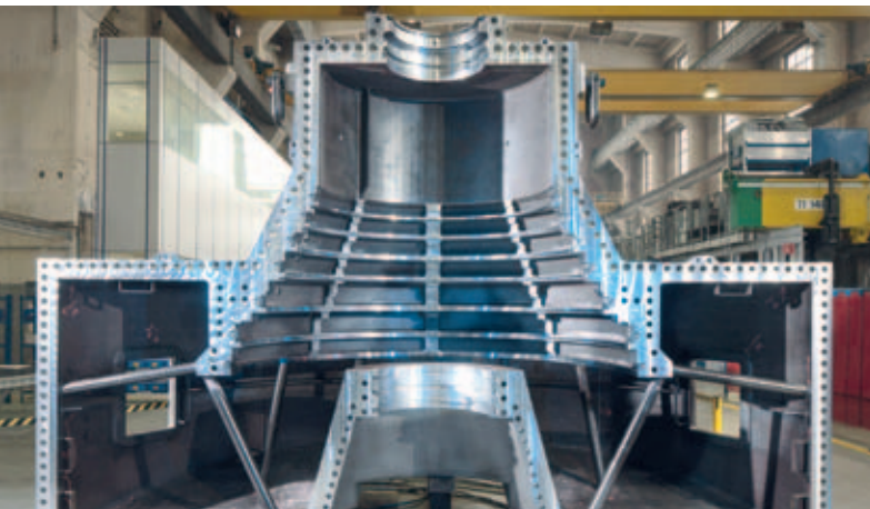
Machining of geothermal steam turbine casing, Siemens facility Goerlitz, Germany.
