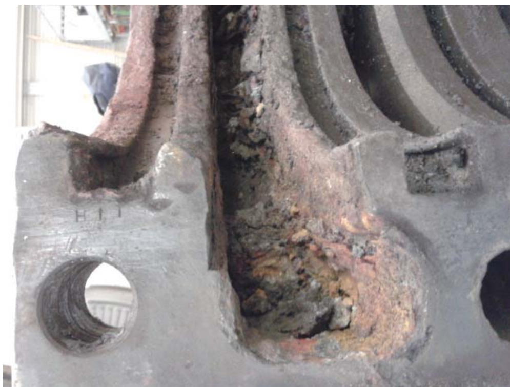
Figure 10. Scaling and corrosion in turbine casing
