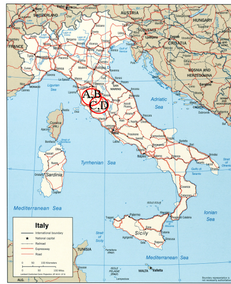
Figure 33: Location of Larderello [A, 594 MW], Travale/Radicondoli [B, 160 MW], Bagnore [C, 20 MW] and Piancastagnaio [D, 68 MW].
