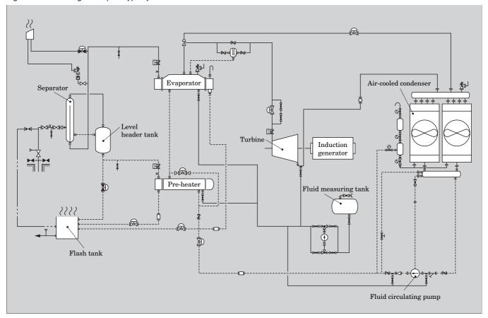
Fig.3 Overview of prototype system
