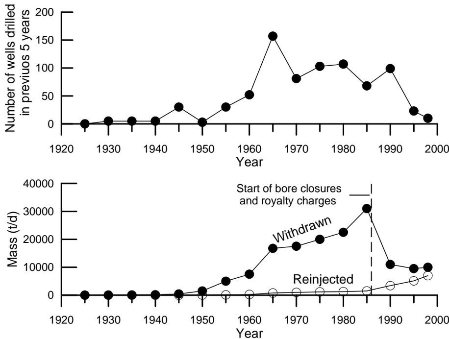
FIGURE 25: History of wells drilled in Rotorua, and the amounts of fluid withdrawn and reinjected; note the rapid decrease in mass withdrawn and increase in mass reinjected following the start of bore closures and imposition of royalty charges. Data from Scott & Cody (2000)
