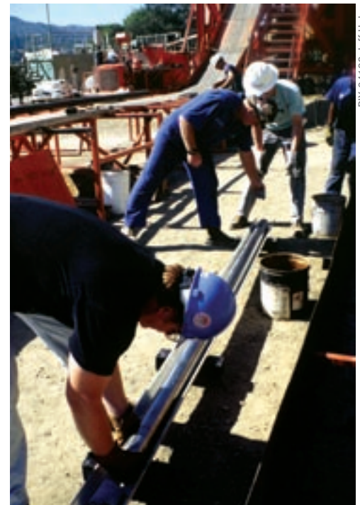
Workers set up a coring rig at The Geysers in Northern California.
