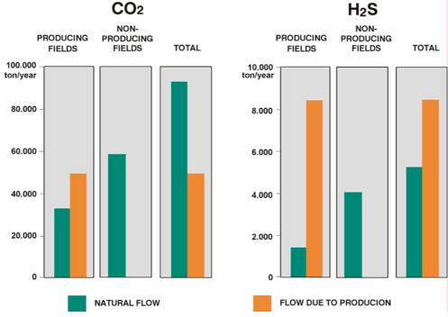
Figure 2 CO<sub>2</sub> and H<sub>2</sub>S emission from producing and non-producing fields
