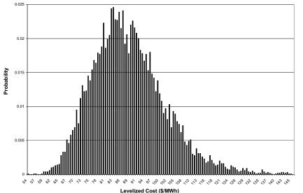
Figure 6. Levelized Cost of a Double-Flash Geothermal Power Plant – Probability Distribution Function.
