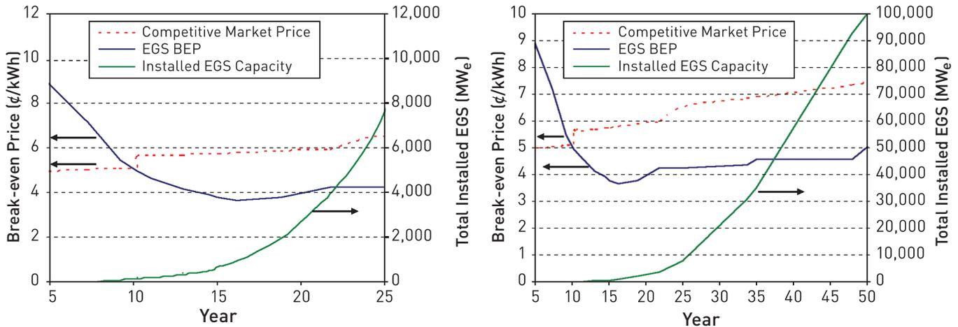
Figure A.9.5 Levelized break-even COE using MIT EGS for the 100,000 MW<sub>e</sub> - 50 year scenario using a fixed charge rate of 12.8% per the NEMS model. Flow rate per production well (in a quartet configuration - 1 injector, 3 producers) follows the 80 kg/s learning curve. Thermal drawdown is 3%/yr resulting in well-field rework after ~ 6 years. Resulting absorbed technology deployment cost is \$262MM U.S. (2004).
