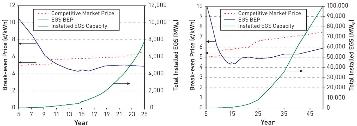
Figure A.9.6 Levelized break-even COE using MIT EGS for the 100,000 MW<sub>e</sub> - 50 year scenario using a fixed charge rate of 12.8% per the NEMS model. Flow rate per production well (in a triplet configuration - 1 injector, 2 producers) follows the 80 kg/s learning curve. Thermal drawdown is 3%/yr resulting in well-field rework after ~ 6 years. Resulting absorbed technology deployment cost is \$344MM U.S. (2004).
