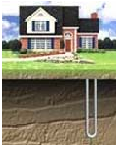
Figure 17 - A Vertical Loop - Alliant Energy
